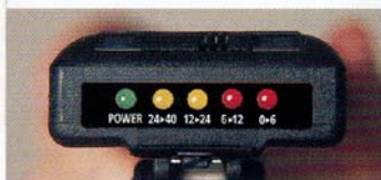
LED display shows you how far away lightning is striking and if the storm is approaching or leaving.
